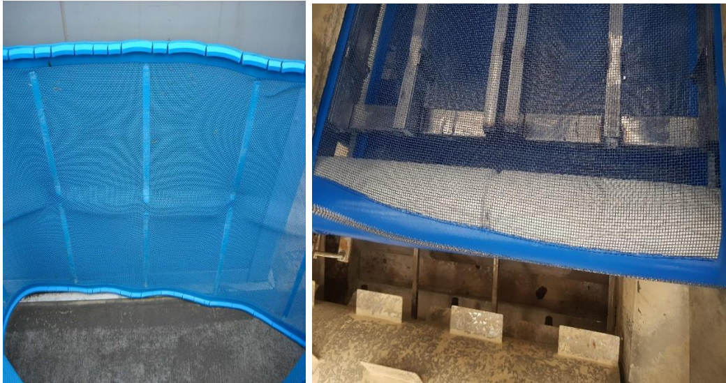
Cracking of v-guides and misalignment of fasteners.
