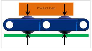
Fig 1 Load is supported totally by uni QNB Balls. No load is supported on the uni QNB links.
