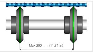
Fig 10 Discs supporting the uni QNB Ball belt on the return section Use discs with a rubber ring to ensure that they will always rotate
