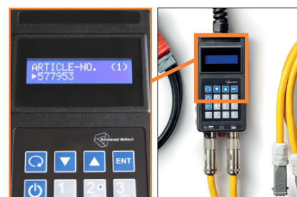
User-friendly control box: simply input the article code number of the belt to be spliced.
