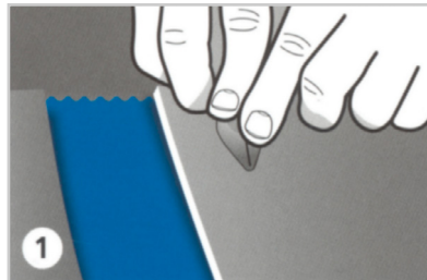
Score the back and lubricate the pin.
