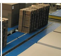
Traditional product removal methods via forklift trucks are no longer the economic option for the modern corrugated board plant, investment in an integrated intelligent handling system incorporating plastic modular belts has become the new standard for the corrugated industry.
