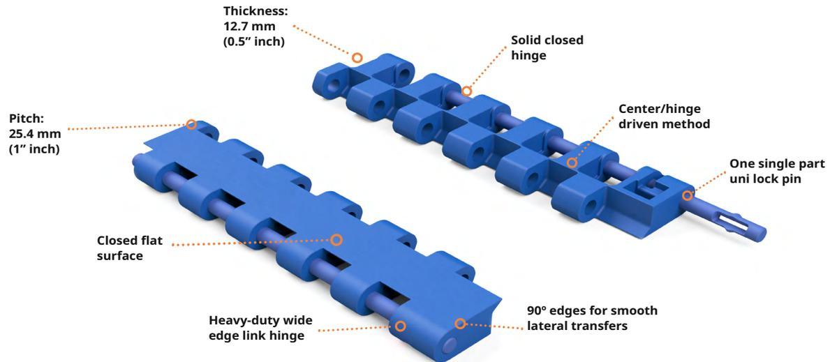
uni ITB width starts from 127.0 mm (5.00 inches), increasing in steps of 25.4 mm (1.00 inch).
