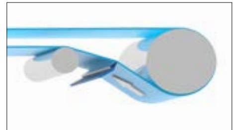
Scraper placement after the drum. Scraper can be placed on the top cover and/or the backside of the belt
