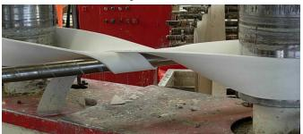
This range of endless woven AmTube Belts provides the best belting solutions to cope with specific and tough conditions found on medium to heavy tube winders.
