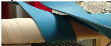
This range of RAPPLON® belts is designed for spiral winding, ensures extremely precise tubes when processing small and medium size tubes.
