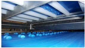
**2) By using the slider bed** Slider bed strips are positioned in such a way that they act as guides for the drive lugs. In this way the belt is self-tracking over the entire slider bed.
