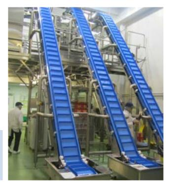
For special applications such as swan necks, the lugs can be positioned on the edges of the belt allowing full control in the critical bend of the conveyor.
