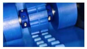
**1) By unique sprocket design** The sprocket's centre piece column also supports tracking and positioning. The belt is fixed in position on the drive and return pulley.
