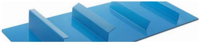
Flat, Angled, Bent all available up to 150 mm high. Smooth finish or profiled using the R18 (positive pyramid) or A18 (inverted pyramid). Made from TPU and using HF welding technology.
