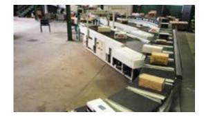
The elastic fabric in STBs makes them suitable to run on pulleys with a strong crowning. Self-Tracking Belts will automatically correct for any effects of pushing, pulling, side loading or other actions that might otherwise result in mistracking issues. These improvements result in less belt damage to belt mistracking and an immediate reduction of maintenance costs.
