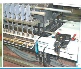
QuickSplice heating pliers with adjustable temperature settings for splicing 110mm fingers as used in the textile industry.
