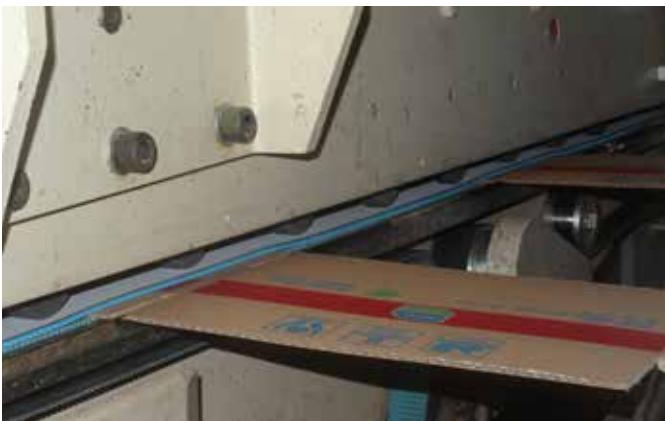
Excellent grip of carton and increased output thanks to wear resistant XNBR Elastomer cover with P6 structure.
