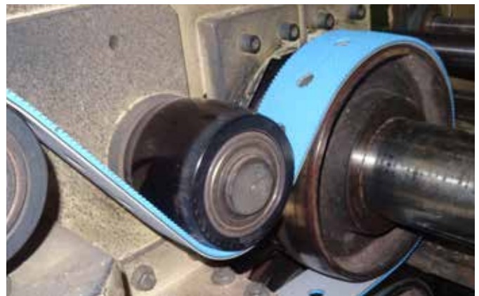
Polyamide foil tensile member offer high flexibility and edge stability.
