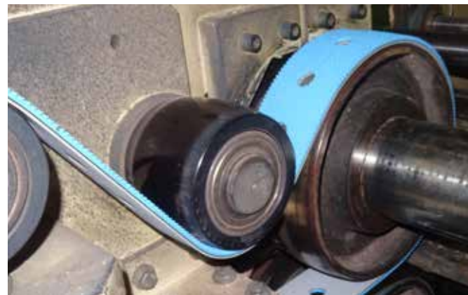
Polyamide foil tensile member offers high flexibility and edge stability.
