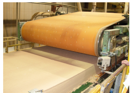
A seamless endless woven prepress belt in action
