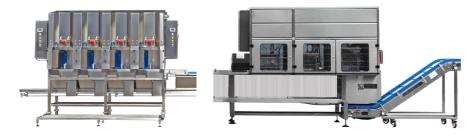
In some cases, it's possible to have a multipurpose machine (for pineapple mainly). The semi-automatic cylinder and coring machine at two heads are suitable for pineapple cylinders. An operator loads the fruit and the machine cuts it in three steps: coring, top and tailing, cylindering.
