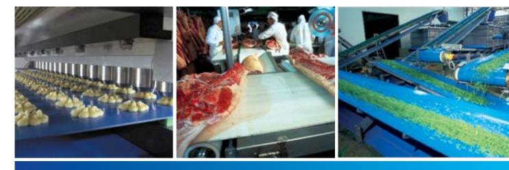
In focusing on hygiene in the food processing industry, Ammeraal Beltech has developed a wide range of AntiMicrobial belting, retaining the well known properties of the regular Food Grade belts. Ammeraal Beltech's AntiMicrobial belting range uses non-migrating materials – a technology based on silver ions. The belt is proven safe for human contact and effective against a broad spectrum of micro-organisms.
