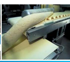
As a leading manufacturer of Process and Conveyor belts for the food industry, Ammeraal Beltech has made food production hygiene a cornerstone of the business. Ammeraal Beltech has developed a reliable protective system to prevent belt edges from soiling and fraying. This also prevents bacteria from penetrating, which is an important step in assuring compliance with ISO 22000 requirements (previously HACCP).
