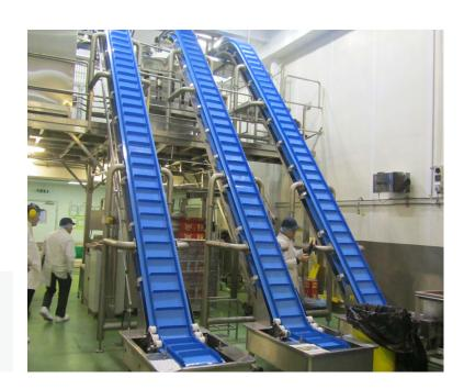
For special applications such as swan necks, the lugs can be positioned on the edges of the belt, allowing full control at the critical bend of the conveyor.
