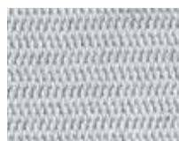
Broken twill weave GK Equally spaced air pockets
