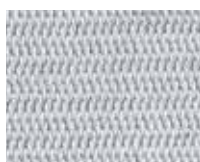
Broken twill weave GK Equally spaced air pockets
