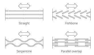
• Fasten only profiles in one end in order to avoid that they bend up in case of temperature rise.
