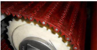
Modular belts are widely used in tyre manufacturing due to their durability, performance, and features like self-tracking and easy installation. However, some manufacturers hesitate to use them in certain stages to prevent the risk of belt fragments causing production interruptions or equipment damage.
