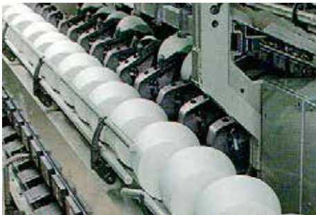
Conveyor belt with smooth belt surface for yarn roll transport.
