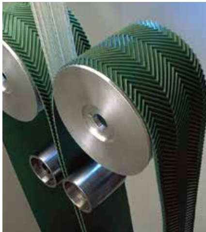
Piddler belt in action during viscose production.
