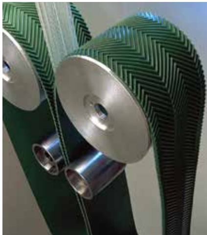
Piddler belt in action during viscose production.
