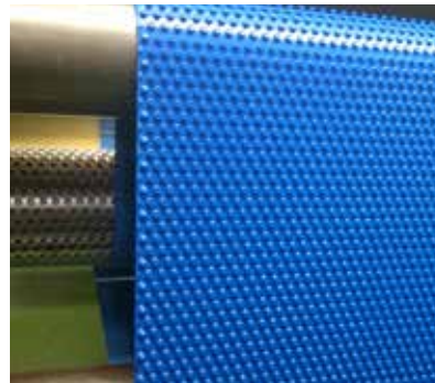
Image of a nipple-profile A17 belt during its profiling process. Customised with a variety of coatings and profiles, the belts are manufactured using a quality-assurance system based on ISO 9001:2008.
