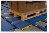
Strength, durability and safety are of paramount concern with floor-level warehouse conveyors, particularly when it may be necessary for employees to step on, off and in between moving belts.
