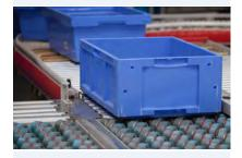
What's more, the RAPPLON range offers two additional advantages – our tangential drive belts offer significant energy savings and lower energy costs, and our Quick-Splice technology eliminates the long downtime required for roller system belt replacement. For roller to roller conveyers, we also offer round belts, which can also be spliced on-site quickly and easily for a minimum loss of time.
