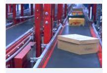
We can offer special profiles and other modifications for increased grip on inclines and declines.
