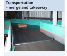
Junctions require narrow tolerances and small drum diameters, but they don't have to be problem spots – Ammeraal Beltech's 45° angled merge belts are perfect for the job and are also resistant to high temperatures.
