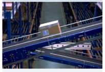
At the heart of the logistics operation, line conveyors often do the bulk of the work. They also consume much of the energy used. Our low runningside coefficient of friction significantly reduces the power required to drive our belts.
