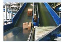
The accumulation stage can be particularly hard on belt longevity. Ammeraal Beltech belting solutions for accumulation are specifically designed to handle the extra wear and tear that occurs during this phase of transportation.
