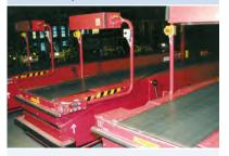
Loading and unloading parcels directly from vehicles with Ammeraal Beltech telescopic conveyor belts simplifies receiving and delivery and it saves time and resources, too. Our telescopic conveyors extend into the vehicle and collapse away after use.
