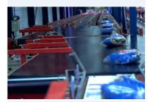
Our belting solutions for accumulation have hard polymer top covers optimized to provide both the ideal surface grip and durability necessary for this stage of the conveying process.
