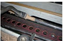
Pletex belts can be hot spliced on site using 'easy to use' QuickSplice tools.
