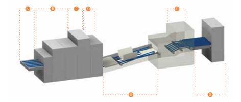
**Counter collector / eject** Demands strong and stable belts with abrasion resistant coatings. A high friction covers guarantees smooth feeding of the cardboard boxes through the counter collector and eject section. Anti-static properties can reduce dust accumulation.
