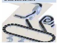
Baggage sorting involves high-speed conyevors equipped with cross-belt and tilt-tray sorters to minimise transfer times.
