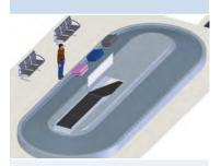
At the final stage of the BHS journey, baggage is delivered to passengers. For transiting passengers, a system is in place to expedite onward baggage transfer.
