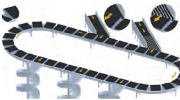
Belt junctions require narrow tolerances and small drum diameters. Our 45° angled merge belts fit the job and are high temperature-resistant.
