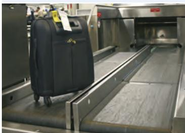
Our belts are **strong** with proven reliability and **feature profiles** designed for the transport of roller-equipped suitcases.
