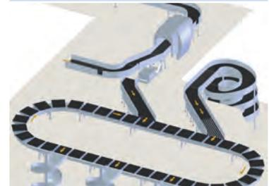
Baggage sorting involves high-speed conveyors equipped with cross-belt and tilt-tray sorters to minimise transfer times.
