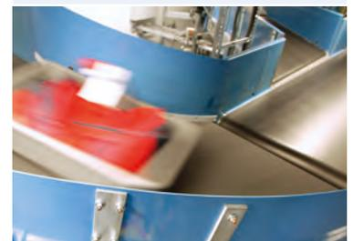
We offer **low noise** belts capable of high-speed power turns. Our extra-strong curve belts can handle loads up to **250 kg**.
