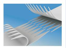
Finger Over Finger (FoF) is the **recommended splicing method** for Flexible Nonex material.
