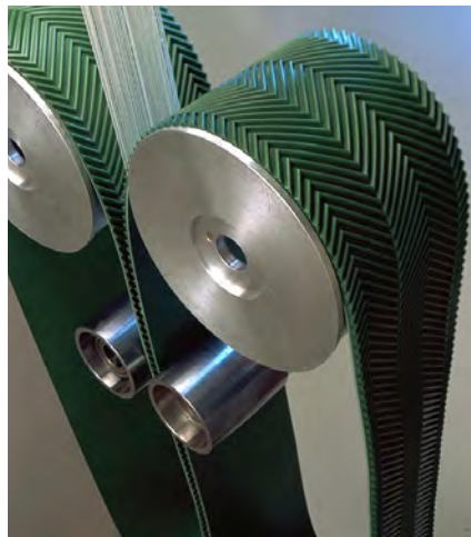
Piddler belt in action during viscose production.
