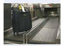
Our belts are **strong** with proven reliability and **feature profiles** designed for the transport of roller-equipped suitcases.
