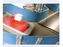
We offer **low noise** belts capable of highspeed power turns. Our extra-strong curve belts can handle loads up to **551 lbs**.
